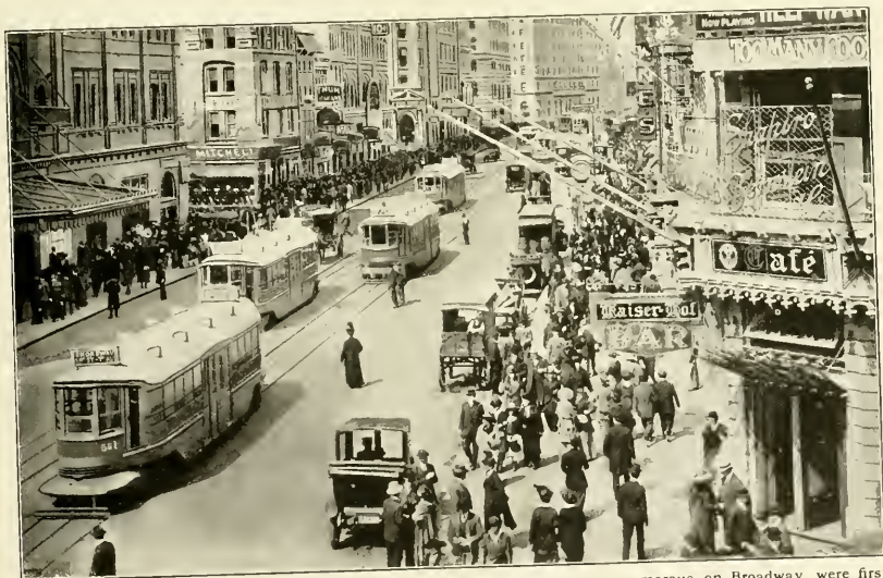
HOBBLE SKIRT CARS, ON BROADWAY —The new surface cars now so numerous on Broadway, were first introduced in 1914. The central portion of the cars is built close to the ground and the doors are in the center of the cars, the steps being only about 6 inches from the ground.
